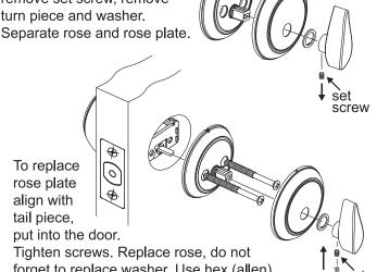
Tighten screws. Replace rose, do not forget to replace washer. Use hex (allen) key to tighten set screw in turn piece.
