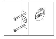
Insert latch and tighten screws.
