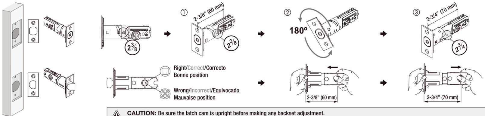
**!** **CAUTION:** Be sure the latch cam is upright before making any backset adjustment.
